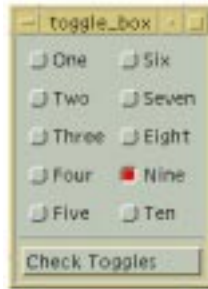
Figure 12-8 Output of the toggle_box program with XmNradioBehavior set True As you can see, simply changing this single RowColumn resource completely changes the appearance of all the ToggleButtons .
